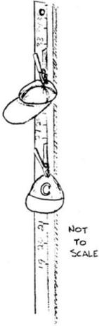
1. Glue one clothespin at each of the 6", 12", 18", 24", and 30" marks. Use either wood glue (for greater strength) or hot glue (for faster drying time) depending on your needs. Body of pins should line up on the centerline of the stick. Jaws should line up with numbers.
