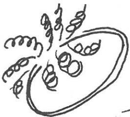
telephone wire ends wrapped around pencil to make coil
