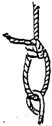
TAUTLINE HITCH FORMS A LOOP WHICH WILL NOT SLIP WHEN ROPE IS TIGHT.
