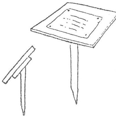
PULPIT SIGN - Made of wood, Good for things close to ground. Easy to read.
