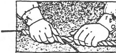
Untwist rope and place wire in the gap.
